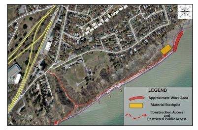
Trucks will access the shoreline via the TRCA access road off of Glen Everest Road east of Wynnview Court and west of Fishleigh Drive. Material will be temporarily stockpiled at the base of the bluffs by the eastern limit of the Fishleigh Drive shoreline access road. The rubble material will be delivered from Monday to Friday from 7:00 am to 5:00 pm, excluding holidays.
