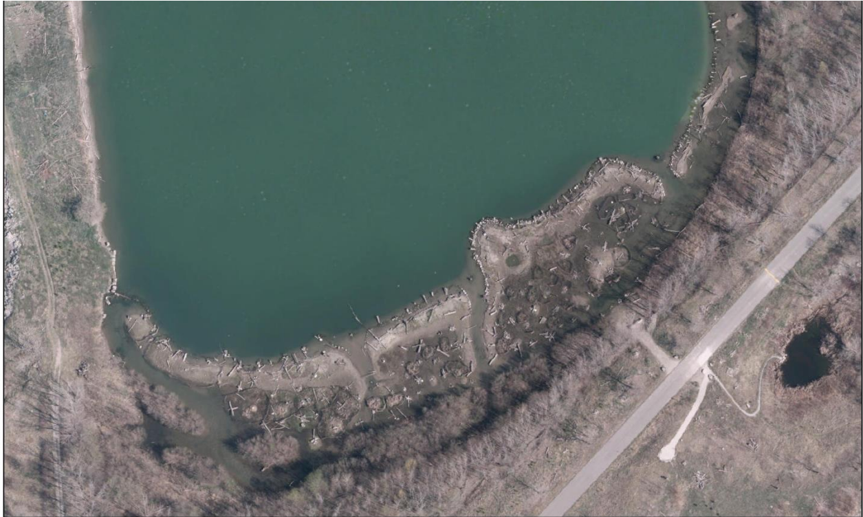
Figure 54: Habitat details immediately post-restoration in Embayment A. These details are typical of the restoration style at Tommy Thompson Park. Fencing can be seen encircling emergent vegetation plots (to protect from waterfowl herbivory), while anchored logs and boulders armour the leeward edges of the newly constructed habitat islands. (City of Toronto 2012)
