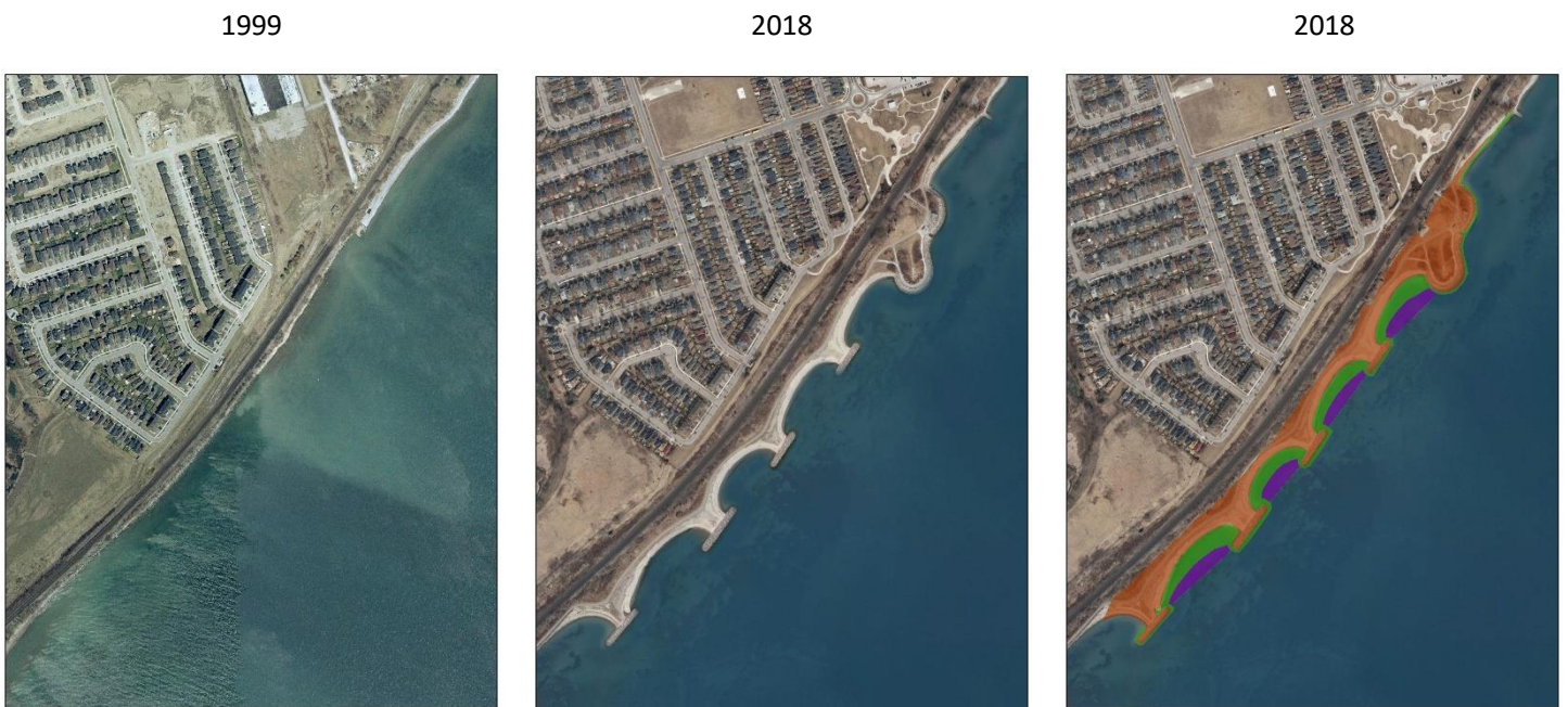
Figure 6: Port Union Phase I project before (left) and after (centre). Project polygons are shown on the far right. (Photos: Triathlon Mapping 1999; City of Toronto 2018).
