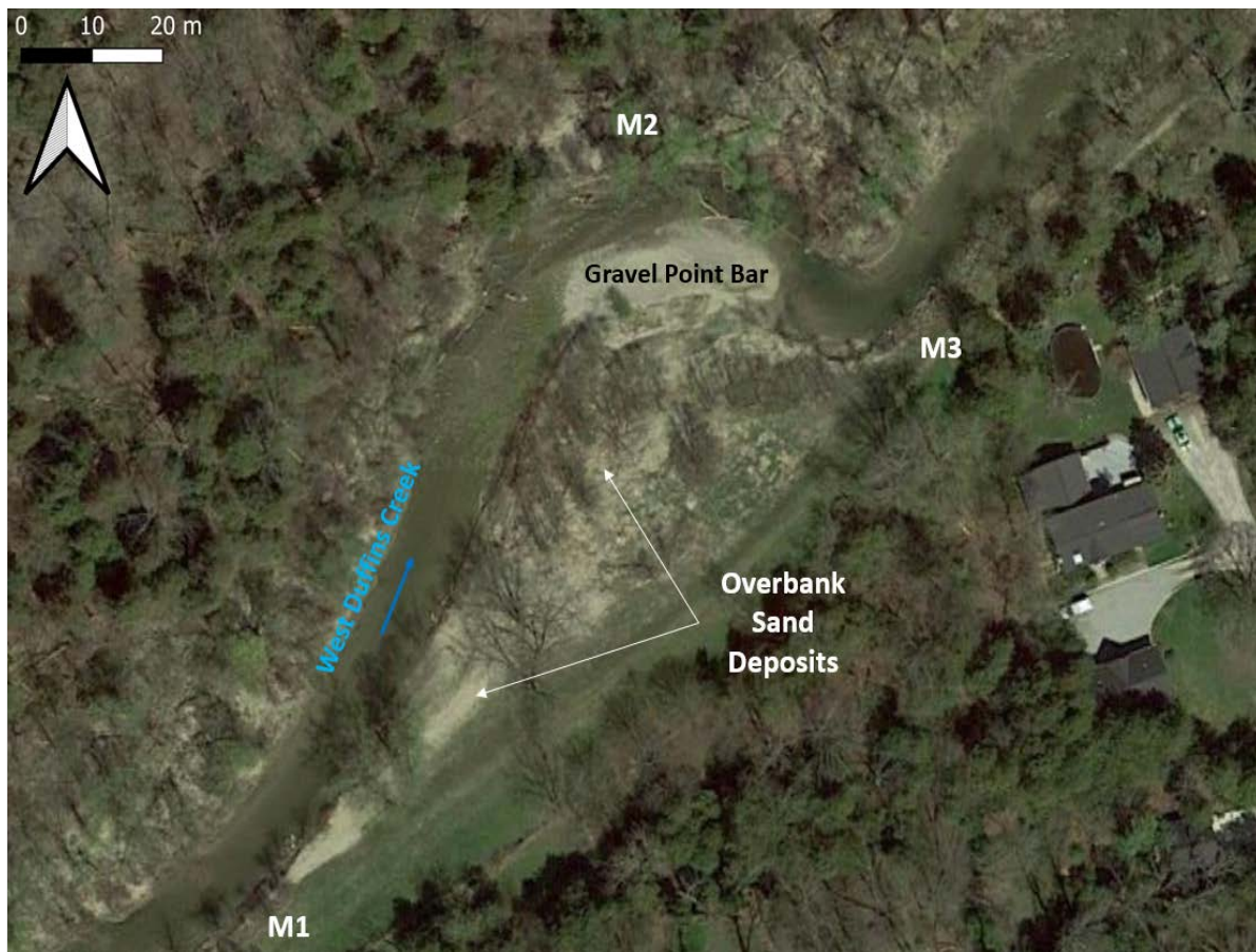
FIGURE: 3-23: OVERBANK SAND DEPOSITION BETWEEN M1 AND M3
