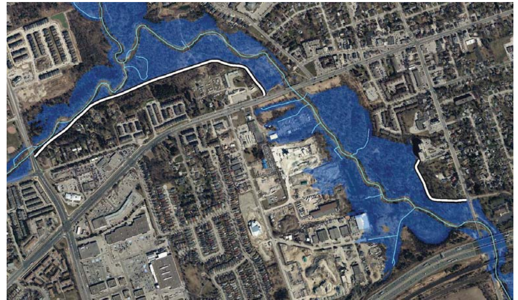
Extent of flooding with proposed dykes
