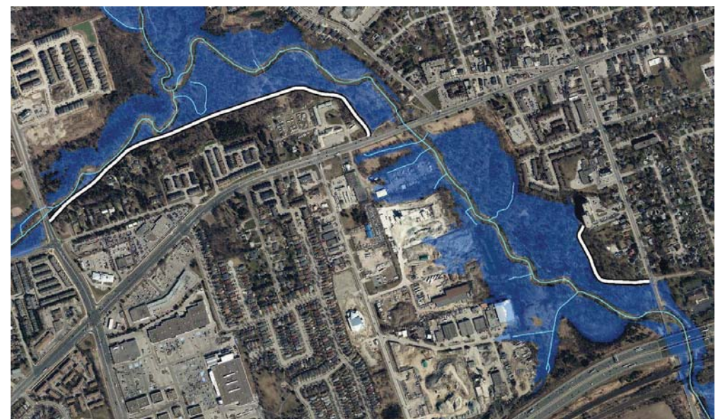
Extent of flooding with proposed dykes
