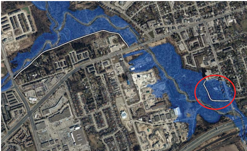
Extent of flooding with current dyke heights
