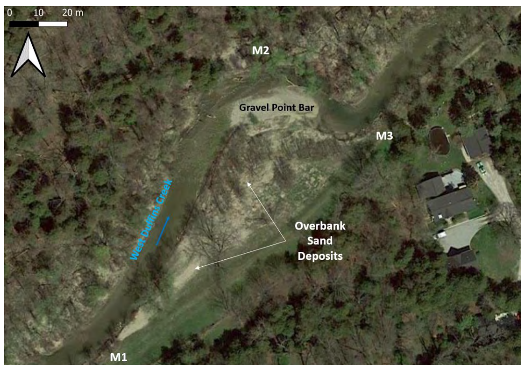
Figure 4. Overbank sand deposition between M1 and M3
