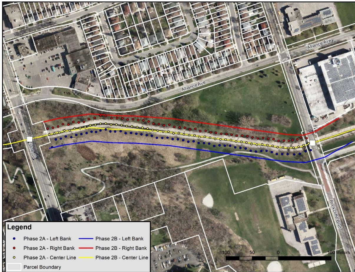
Figure 5.1. Black Creek Channel Widened from Rockcliffe Blvd to Jane St
