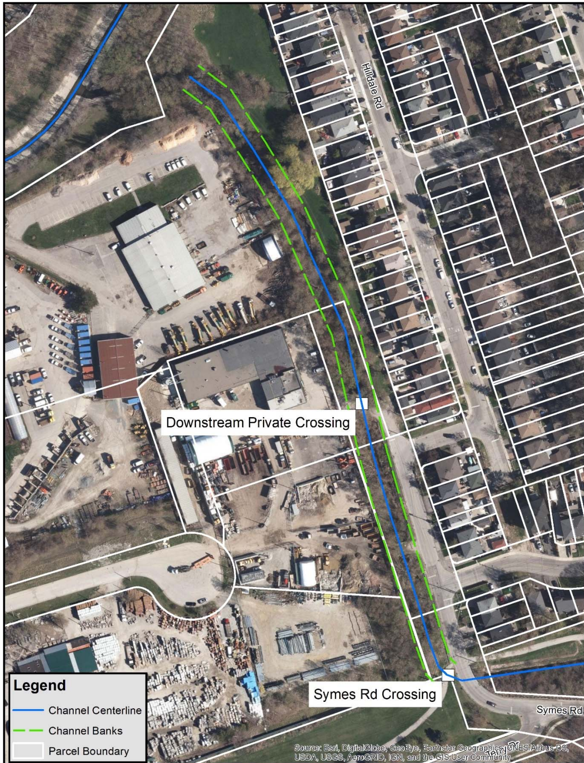
Figure 5.5. Lavender Creek Widened from Symes Road Crossing to Black Creek, 15 m Wide Concrete Channel
