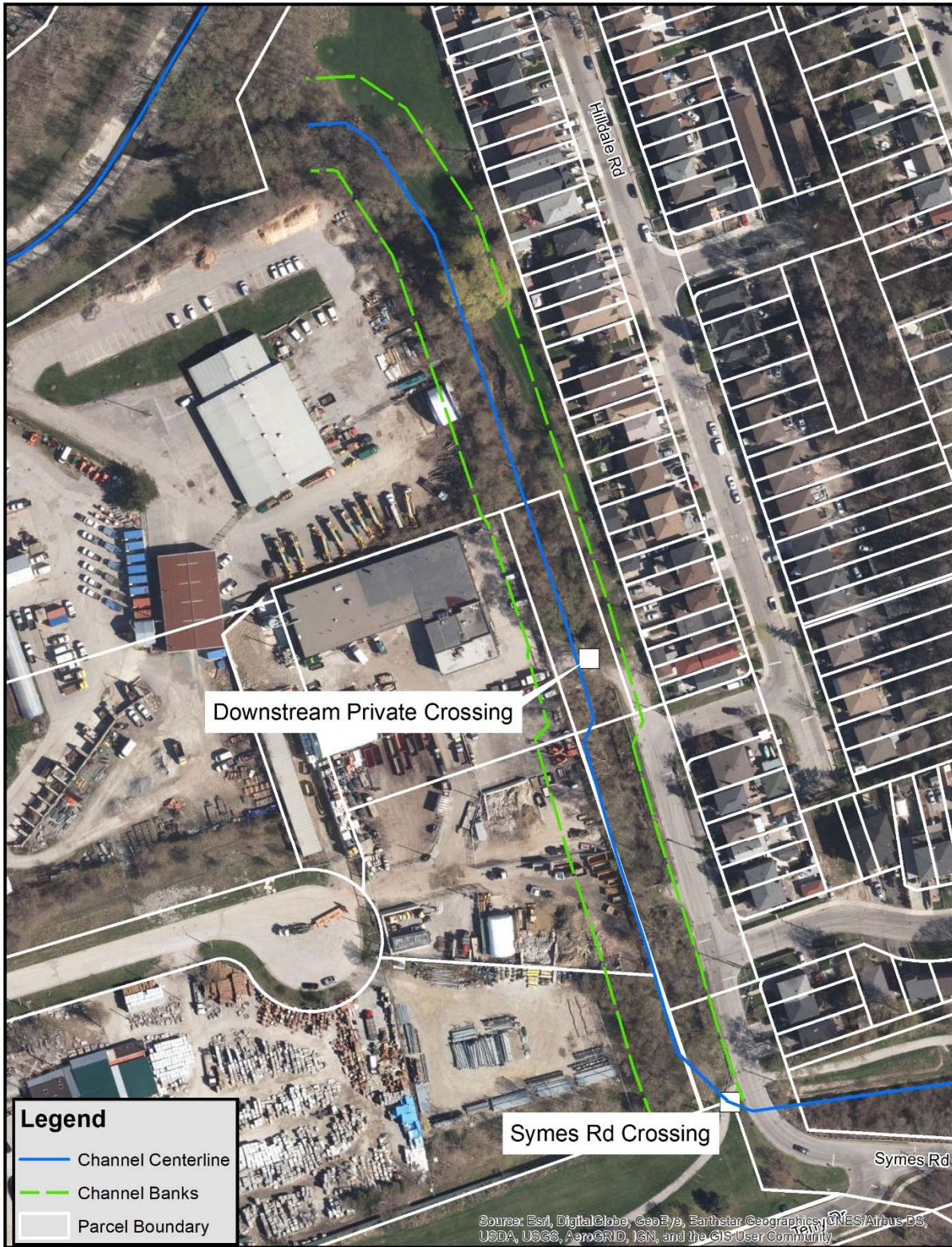
Figure 5.10. Lavender Creek Widened from Symes Road Crossing to Black Creek, 30 m Wide Natural Channel
