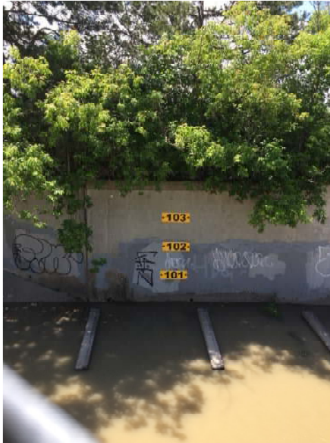
Photo 13 – Flow depth gauge
