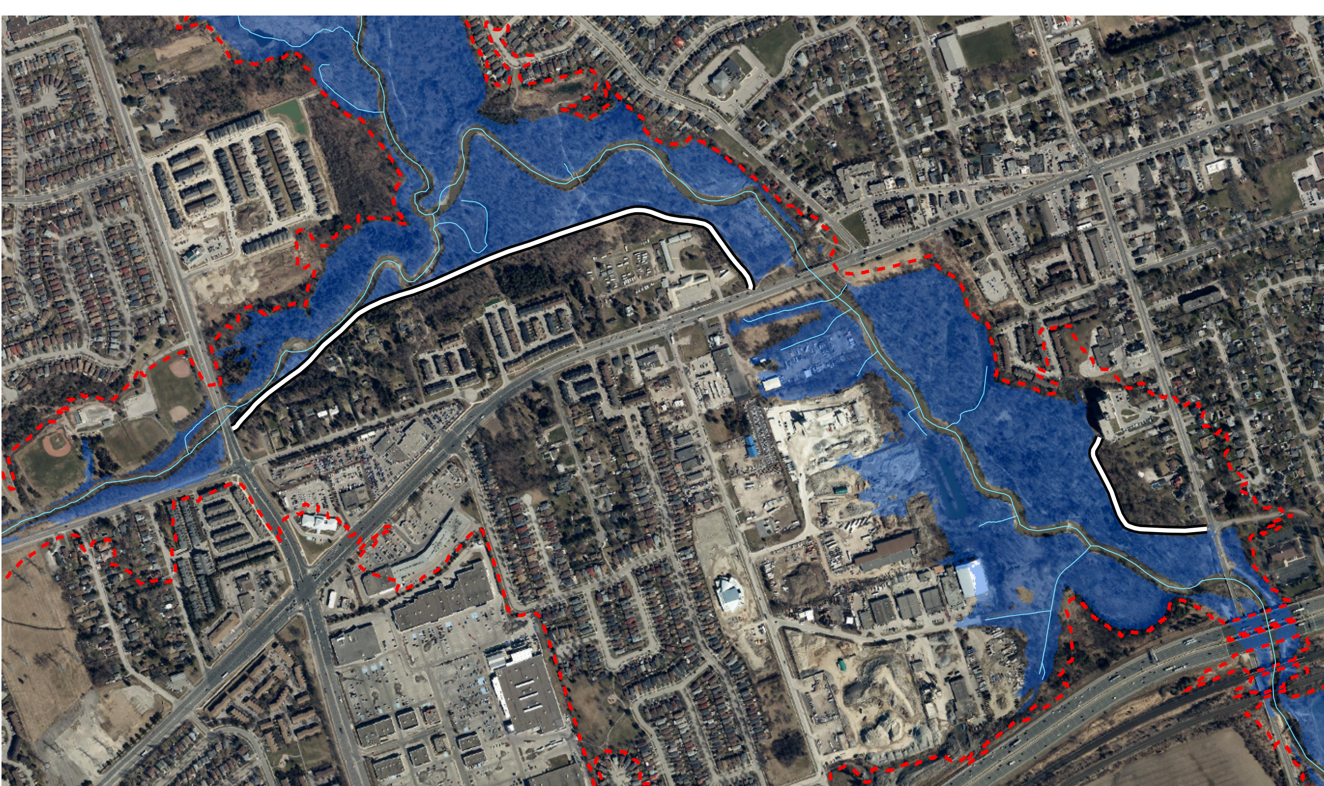
Extent of flooding with proposed dykes
