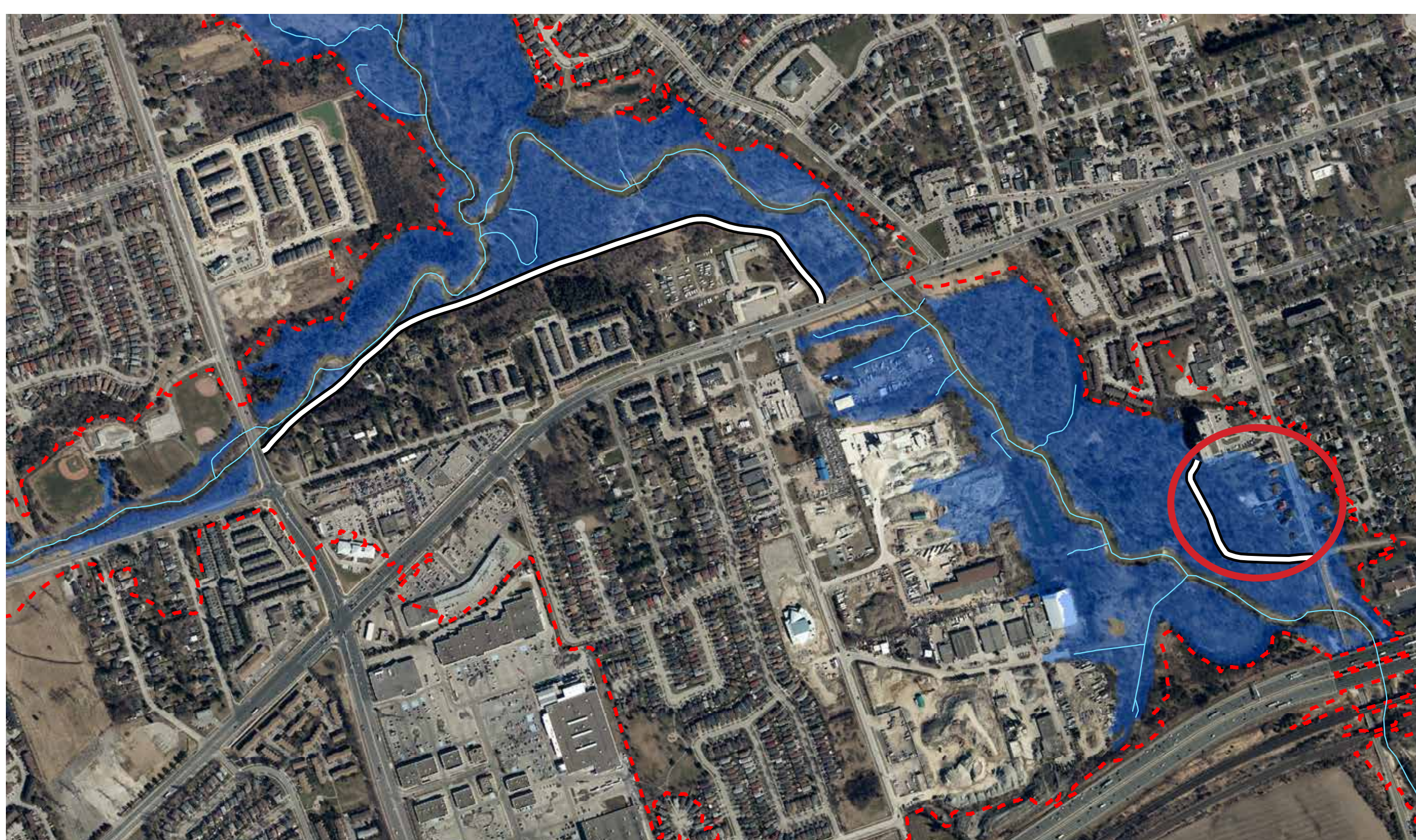
Extent of flooding with current dyke heights
