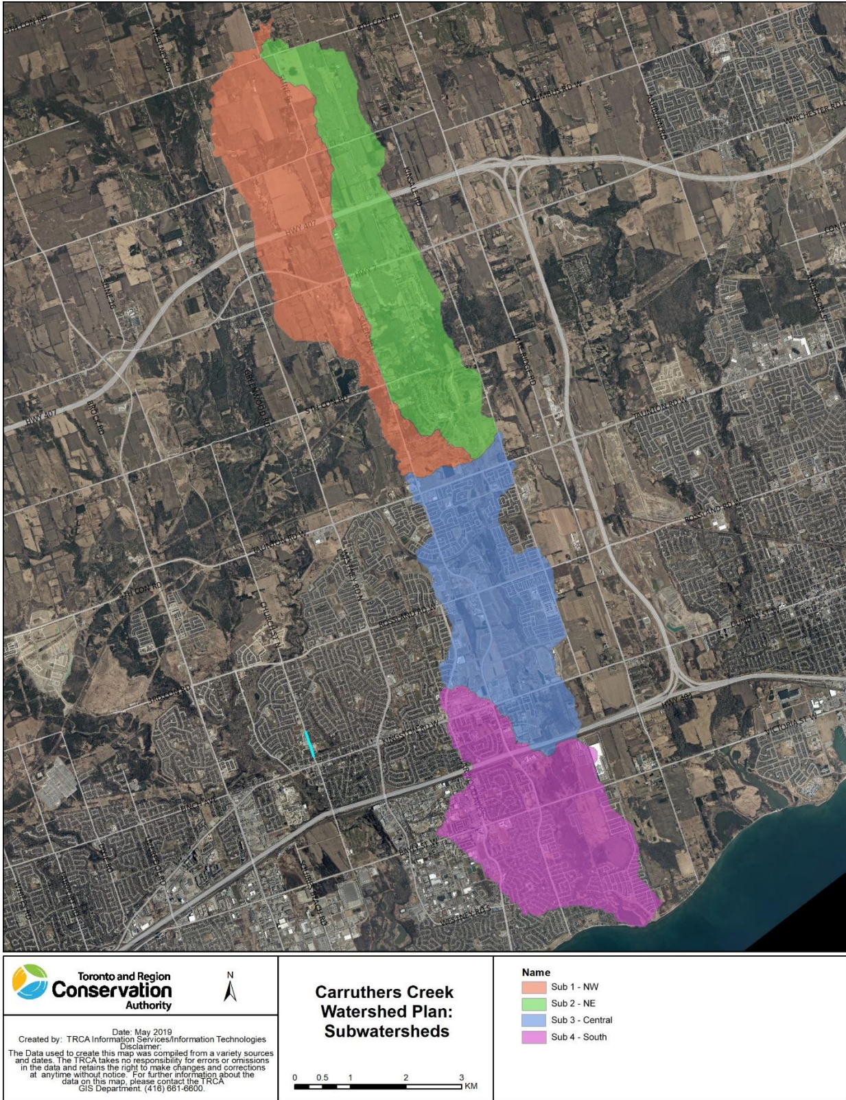
FIGURE 12 THE FOUR SUB-CATCHMENTS (NW, NE, CENTRAL, SOUTH) OF THE CARRUTHERS CREEK WATERSHED USED IN THE SWAT MODEL.
