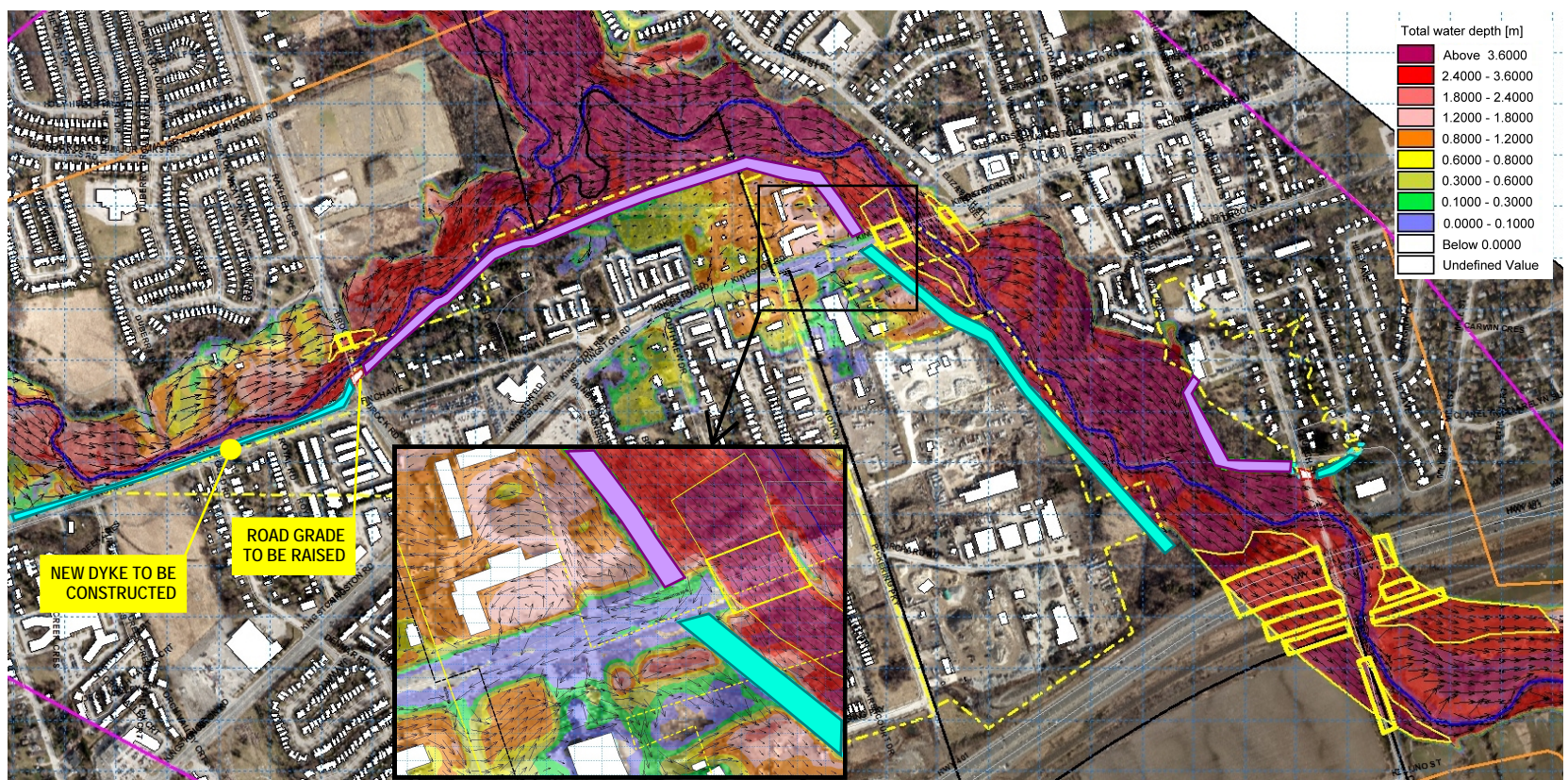
Fig 4.5b Widening Bridges and Channel, Raise Existing Dykes, Construct Three New Dykes, Grade raise at Church and Brock
