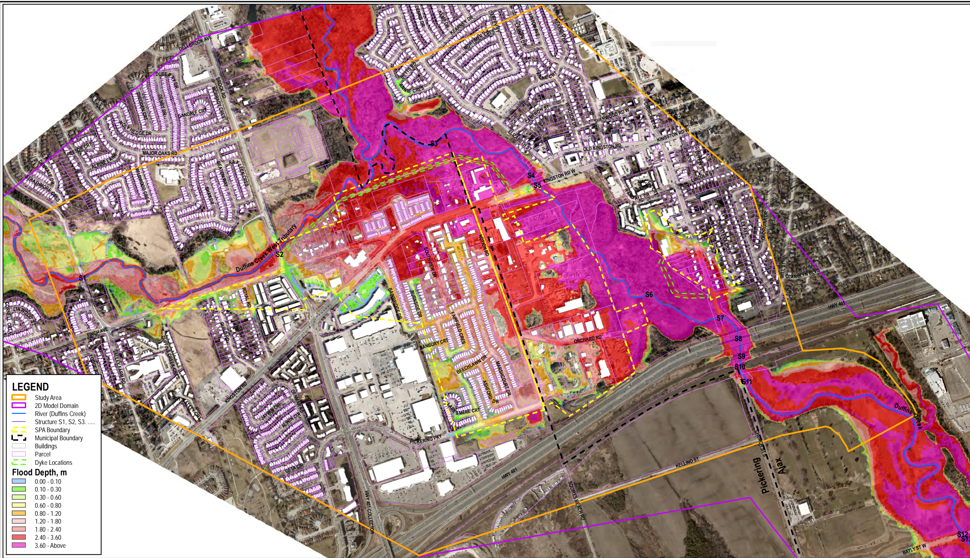
FIGURE 1.3 REGIONAL FLOOD DEPTH MAP ( EXISTING CONDITION )
