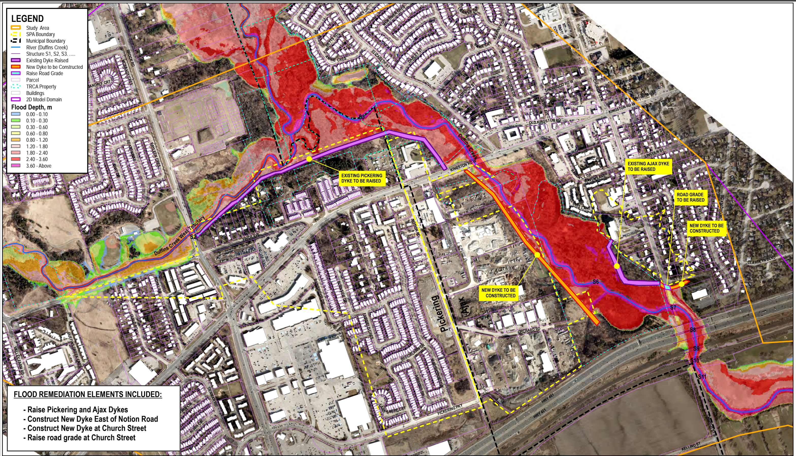
FIGURE 4.2 OPTION 1 : FULL FLOOD REMEDIATION ( 500 - YR ) 500 - YR FLOOD DEPTH MAP STEADY INFLOW HYDROGRAPH ( 500 - YR STORM )
