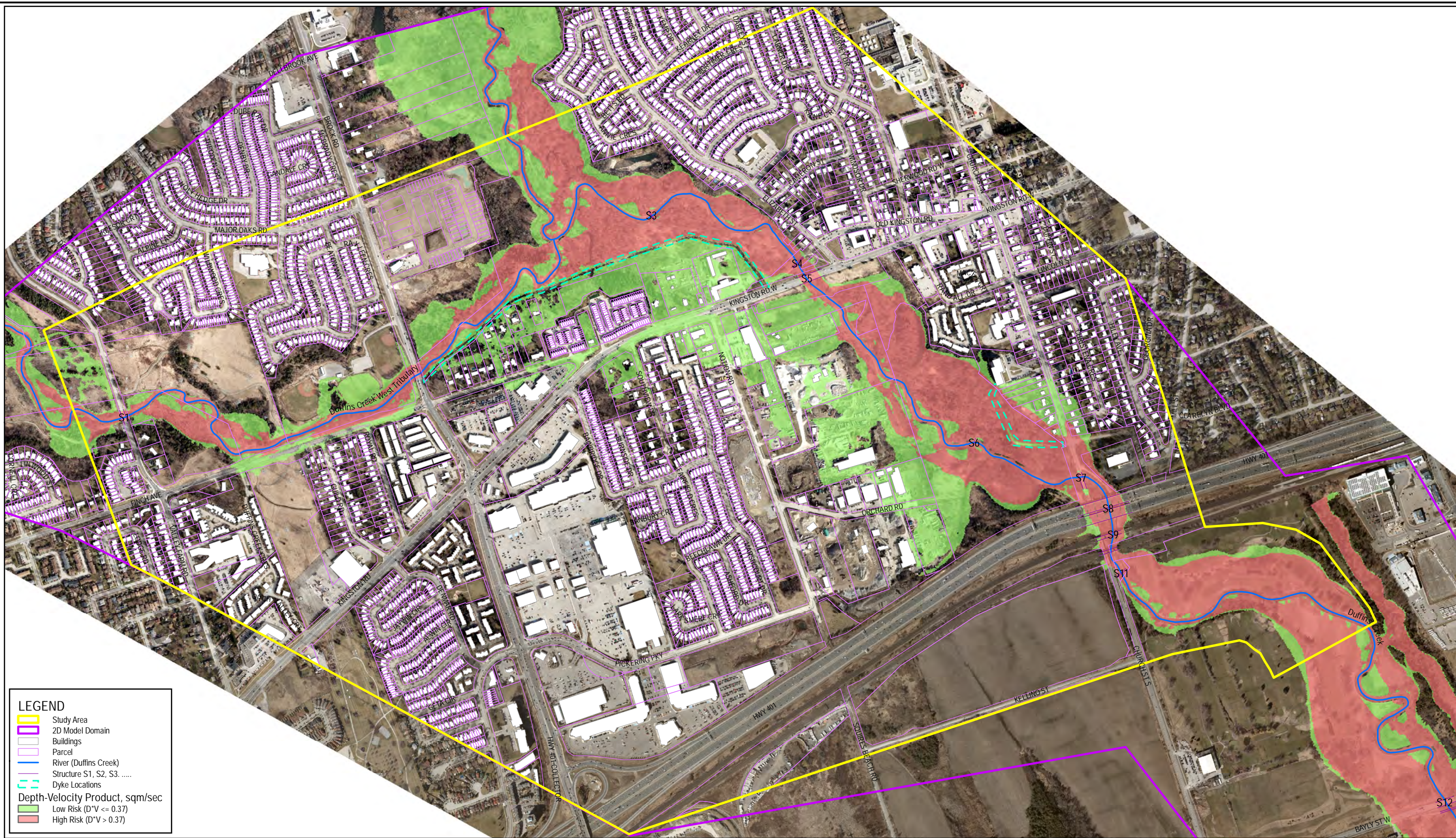
Figure E.19 350-YR DEPTH-VELOCITY PRODUCT MAP (EXISTING CONDITION) STEADY INFLOW HYDROGRAPH (350-YR STORM)
