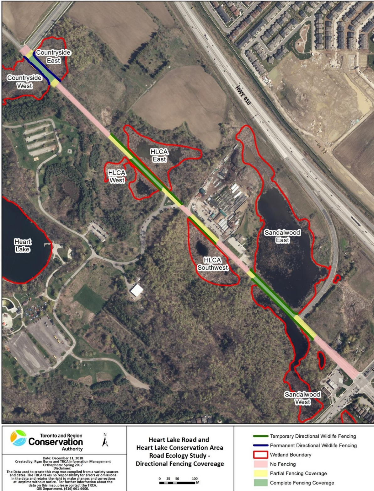
FIGURE 11. COMPLETE, PARTIAL AND NO FENCE COVERAGE ALONG HEART LAKE ROAD IN 2018.
