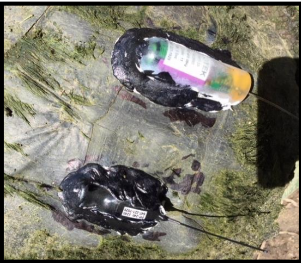
FIGURE 6. VHF (WHITE) AND GPS UNIT (BLACK) ATTACHED TO THE MIDDLE OF THE CARAPACE OF A SNAPPING TURTLE.
