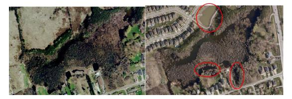
**FIGURE 4.5:** Snively wetland, Richmond Hill. Photo on the left was taken in 2002 prior to development. Photo on the right shows the wetland in 2009 following development to the northwest. Note the stormwater management pond, and areas with obvious shifts in vegetation circled in red.
