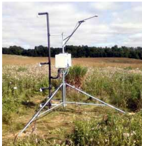
Figure 44: Automated Bowen Ratio Energy Balance system used to determine “actual” evapotranspiration values, located at Kortright Conservation Area.
