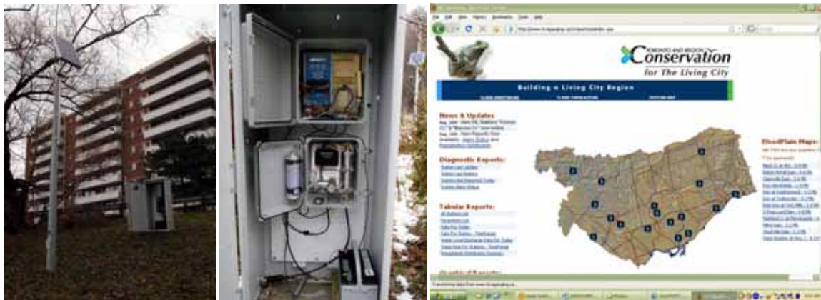
Figure 33: Various RT stream gauge stations (from left) Taylor Massey Creek, McFall Dam, and the RT gauging home page.
